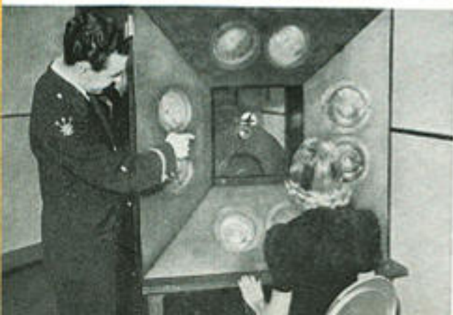
Outmoded mechanical scanning camera. Subject sat before photoelectric cells.
