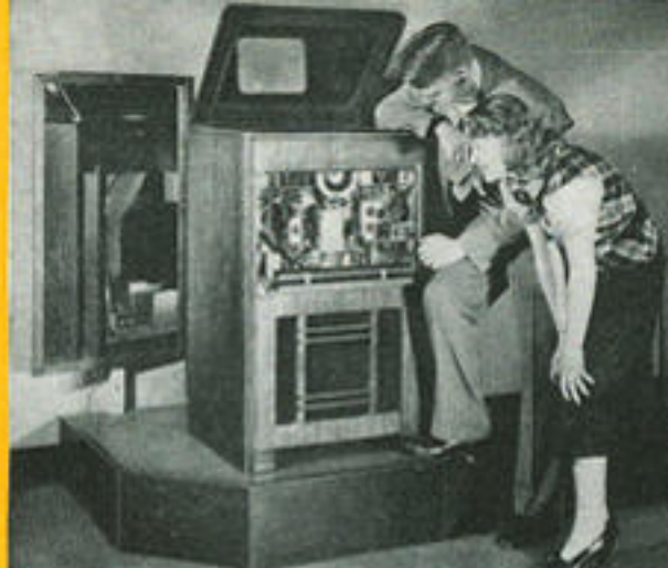
RCA television receiver with front panel removed to show the interior.
