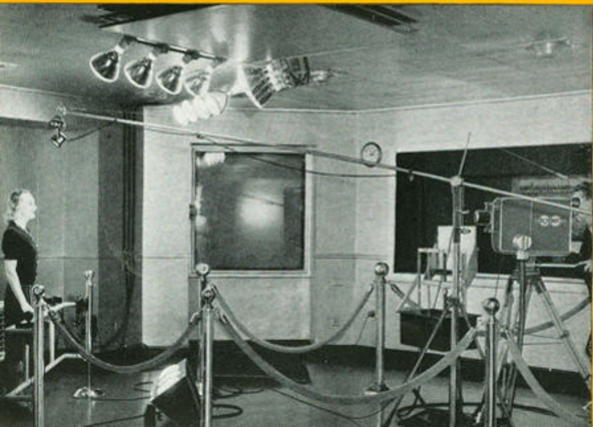
Interior of the Tour television studio, showing how a guest is televised. The camera operator is at the extreme right. The microphone is suspended over the subject's head.
